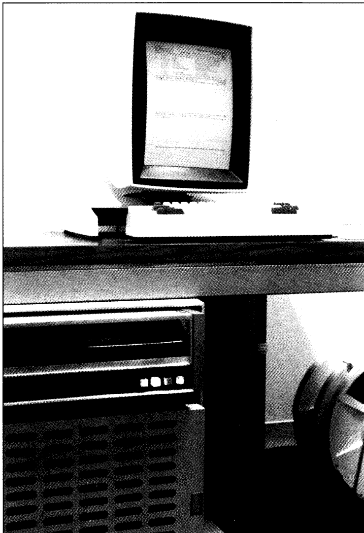
Figure 9. The Xerox Alto. The Alto, developed at Xerox PARC in the seventies, was a prototype for Star. Both its hardware design and the many programs written for it by PARC researchers strongly influenced Star's designers.
